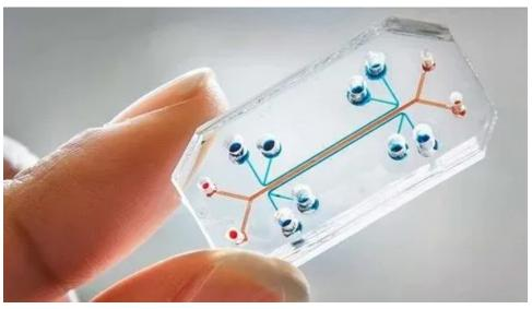
Microfluidics is the technology to manipulate small amounts of fluid using tiny channels, sealed devices, valves, connectors, etc. There are many applications of Microfluidics within research such as cancer cell research, drug testing, organ on a chip, etc. It helps to save reagents in lab, achieve
